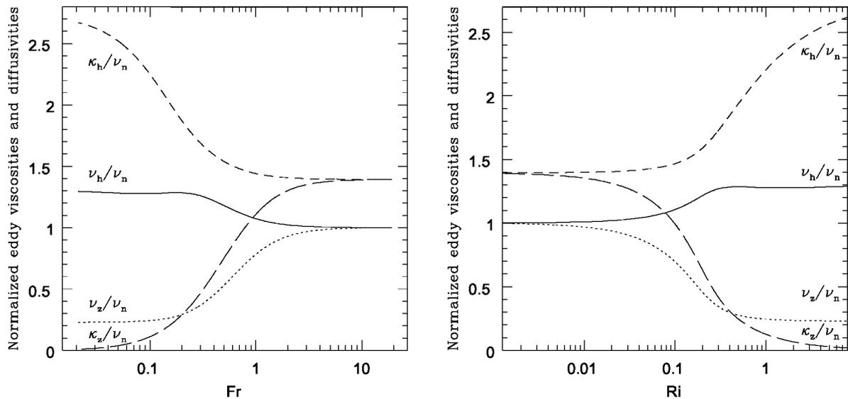
FIG. 1 – Normalized eddy viscosities and diffusivities as functions of the Froude number  $Fr$  (left panel) and the gradient Richardson number  $Ri$  (right panel).
