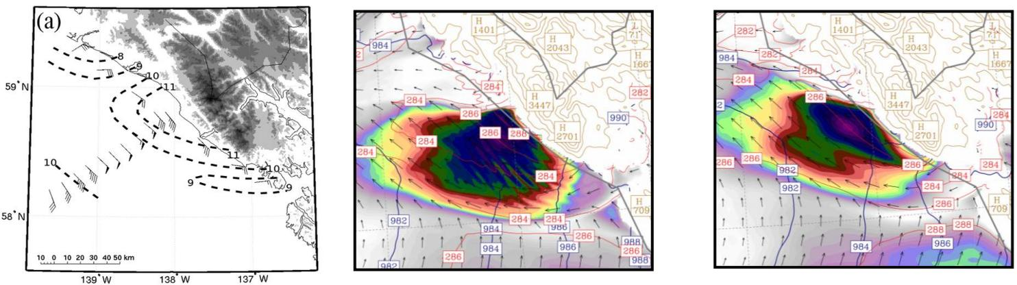
Fig.1 Observed and modeled velocity in barrier jet at 150 m AGL from IOP7 during SARJET field experiment. MYJ on the left, MYNN on the right. From Olson (2008).
