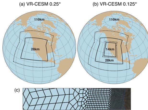
Figure 2. Illustration of grid spacing in the (a) VR-CESM 0.25° and (b) VR-CESM 0.125° meshes. (c) A depiction of the transition from the global 1° resolution mesh through two layers of refinement to 0.25° and again to 0.125° (Huang et al., 2016).
