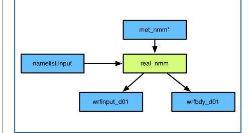
The *real\_nmm.exe* program is used to vertically interpolate the global model data to the WRF levels
