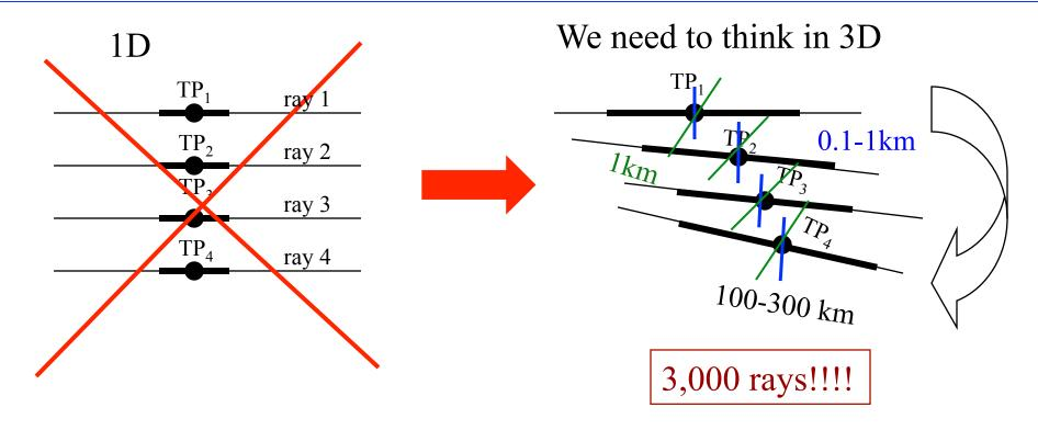
An occultation is not just a vertical profile. The relative motion of the satellites involves an inclination away from the vertical of the surface swept out by the occulting rays (a surface, moreover, that is not in general even a plane)
