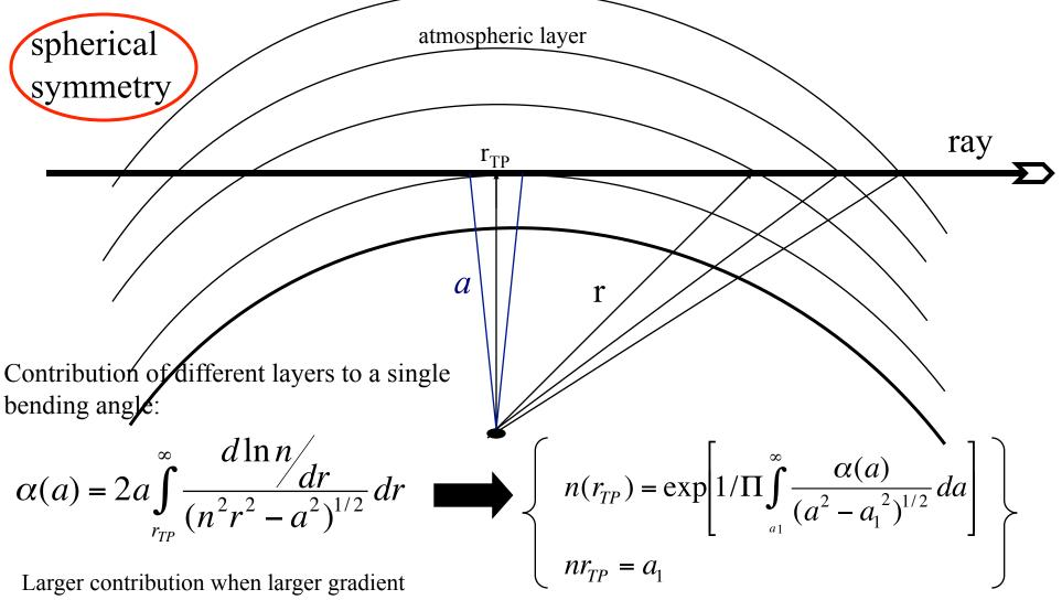
Larger contribution when larger gradient and closer to  $r_{TP}$  -> integral peaks at  $r_{TP}$
